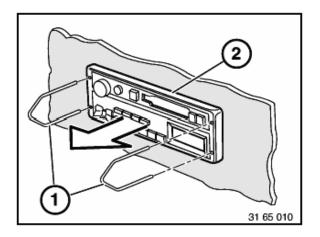
Press unlocking hooks (1) into radio on left and right sides. Pull out radio carefully with hooks.
